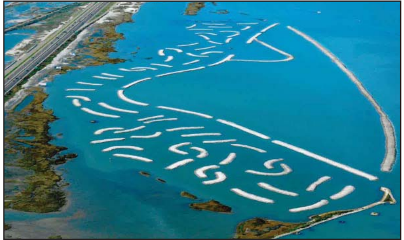
The first phase, seen here in March 2011, created terraces and an outer berm. A second phase will create additional marsh complex in the middle.
