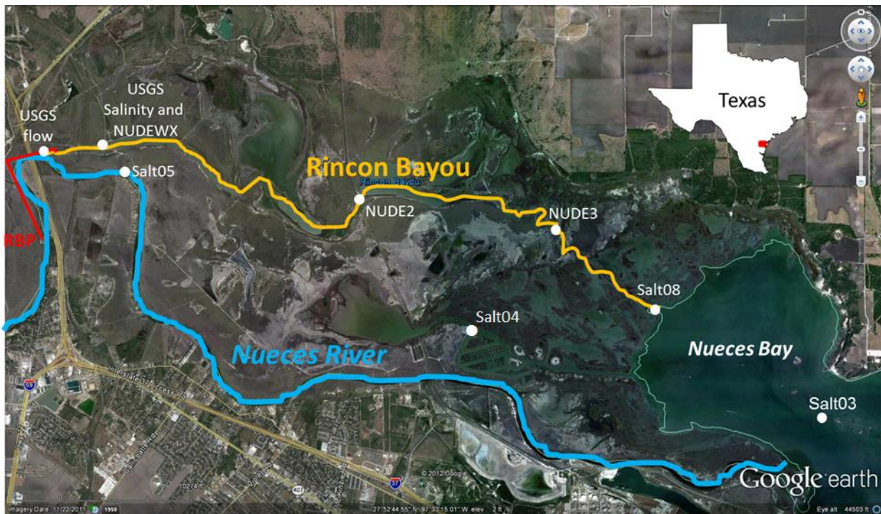
Figure 3. Map showing the RBP (Rincon Bayou Pipeline [red line]) and the four salinity monitoring stations for this project (NUDE2, NUDE3, SALT04, and SALT08).
