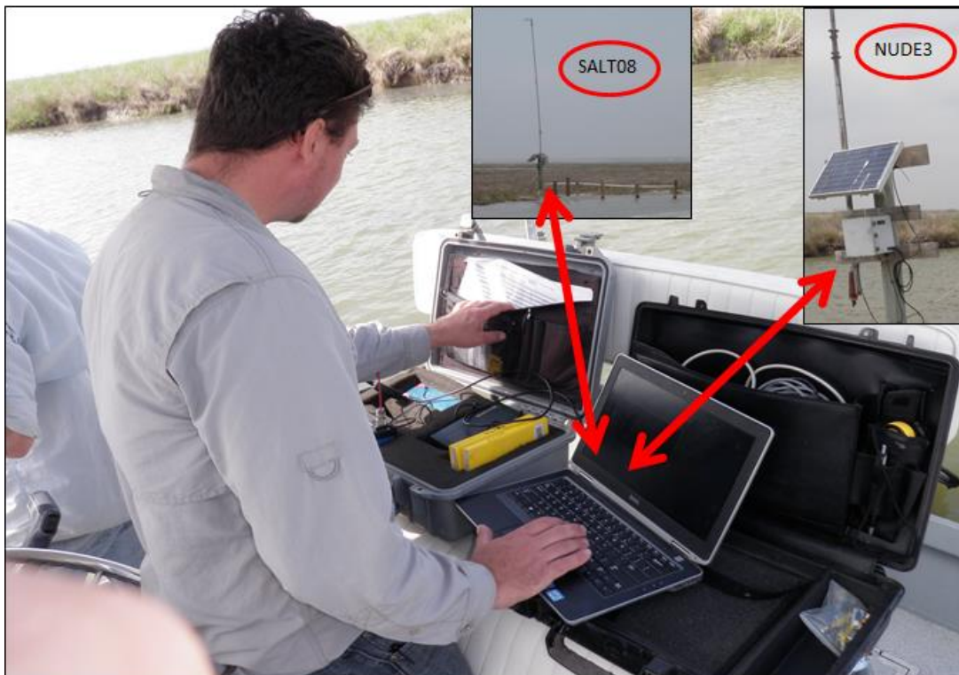
Figure 4. Dominic Burch uses a radio and computer to call NUDE3 and SALT08 before and after exchanging the datasondes to ensure the devices are measuring salinity accurately.
