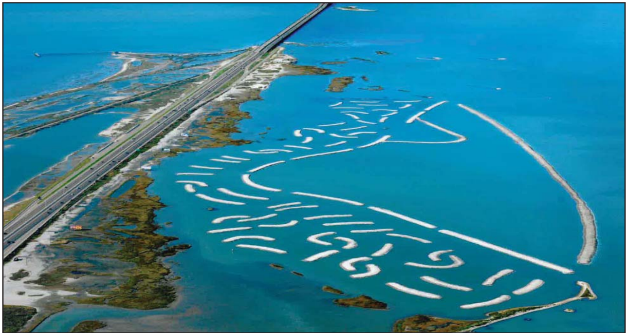
This aerial photo from March 2011 shows the terraces and berms created during the first phase of marsh restoration. A second phase will create additional marsh complex between the terraces and the top berm.
