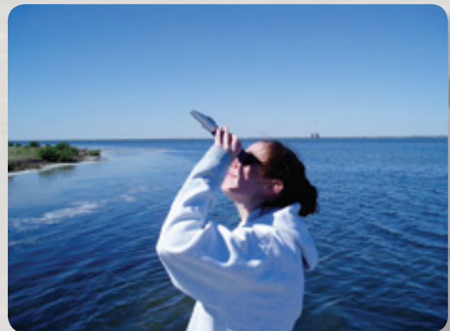
Measuring salinity using a refractometer.
