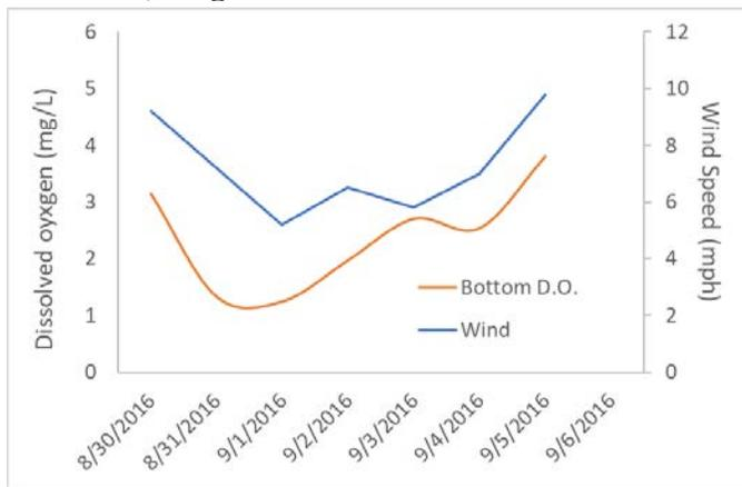
**Figure 12. Relationship between wind speed and bottom water dissolved oxygen. From CM 36, August-September 2016.**
