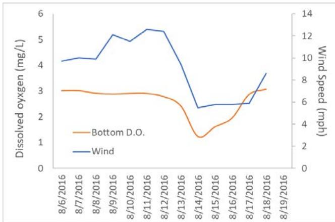
**Figure 11. Relationship between wind speed and bottom water dissolved oxygen. From CM 36, August 2016.**
