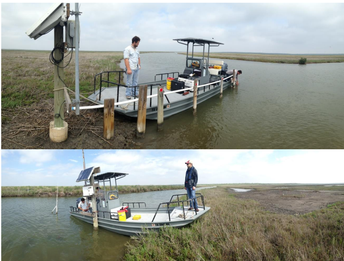
Figure 5. SALT08 (top image) and NUDE3 (bottom image) datasondes are being exchanged with a newly calibrated datasonde which will remain deployed for approximately 4 weeks after which the datasonde will be replaced in the same fashion.
