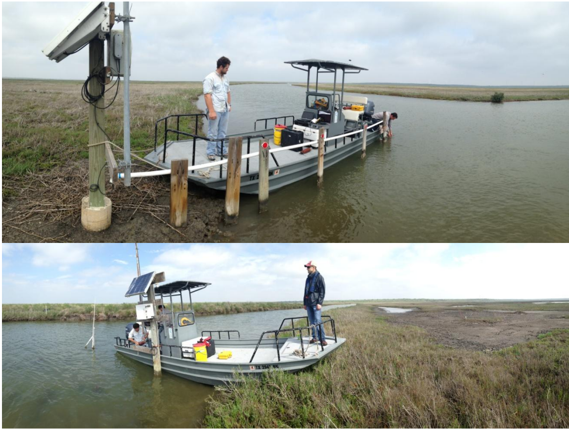
Figure 5. SALT08 (top image) and NUDE3 (bottom image) datasondes are being exchanged with a newly calibrated datasonde which will remain deployed for approximately 4 weeks after which the datasonde will be replaced in the same fashion.
