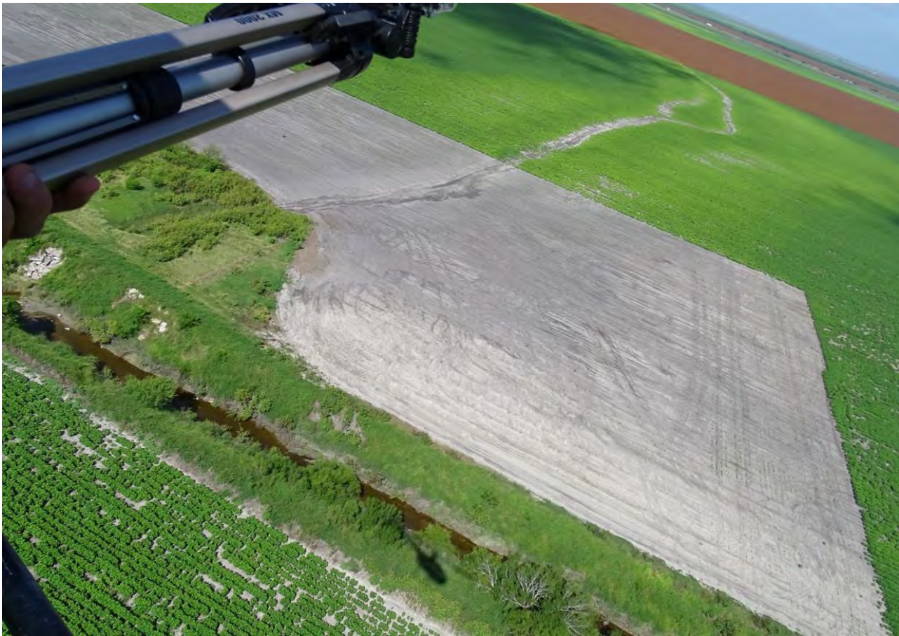
Figure 69 This image shows gullies forming where runoff drains from adjacent farmland into the ditch. Allowing the drain to develop energy dissipating vegetation could slow the runoff and help slow the gully formation.
