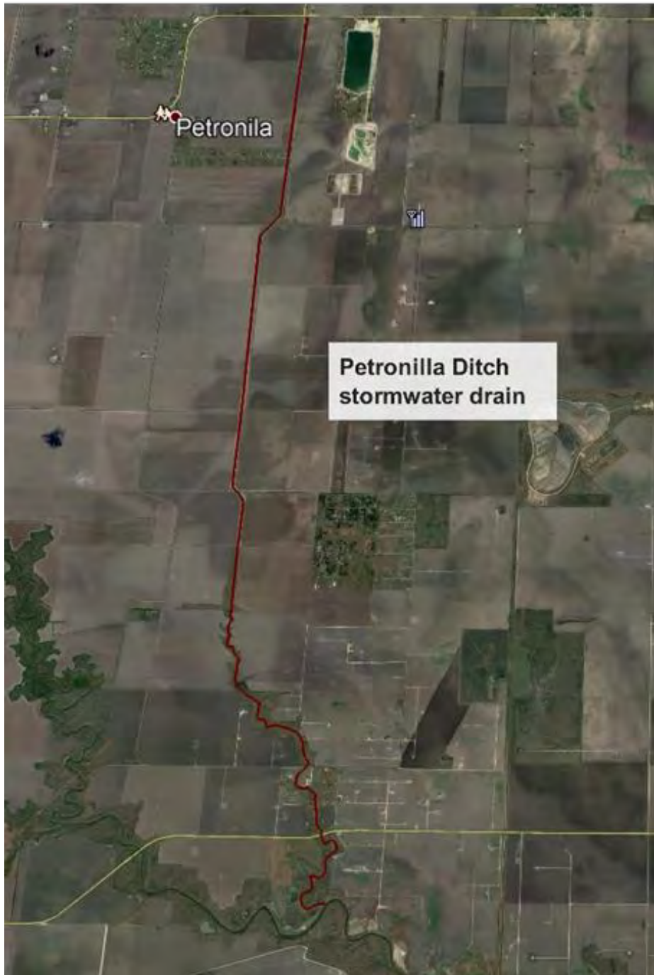
Figure 66 GoogleEarth™ image of the Petronilla Ditch, storm drain to Lower Petronilla Creek highlighted in red.
