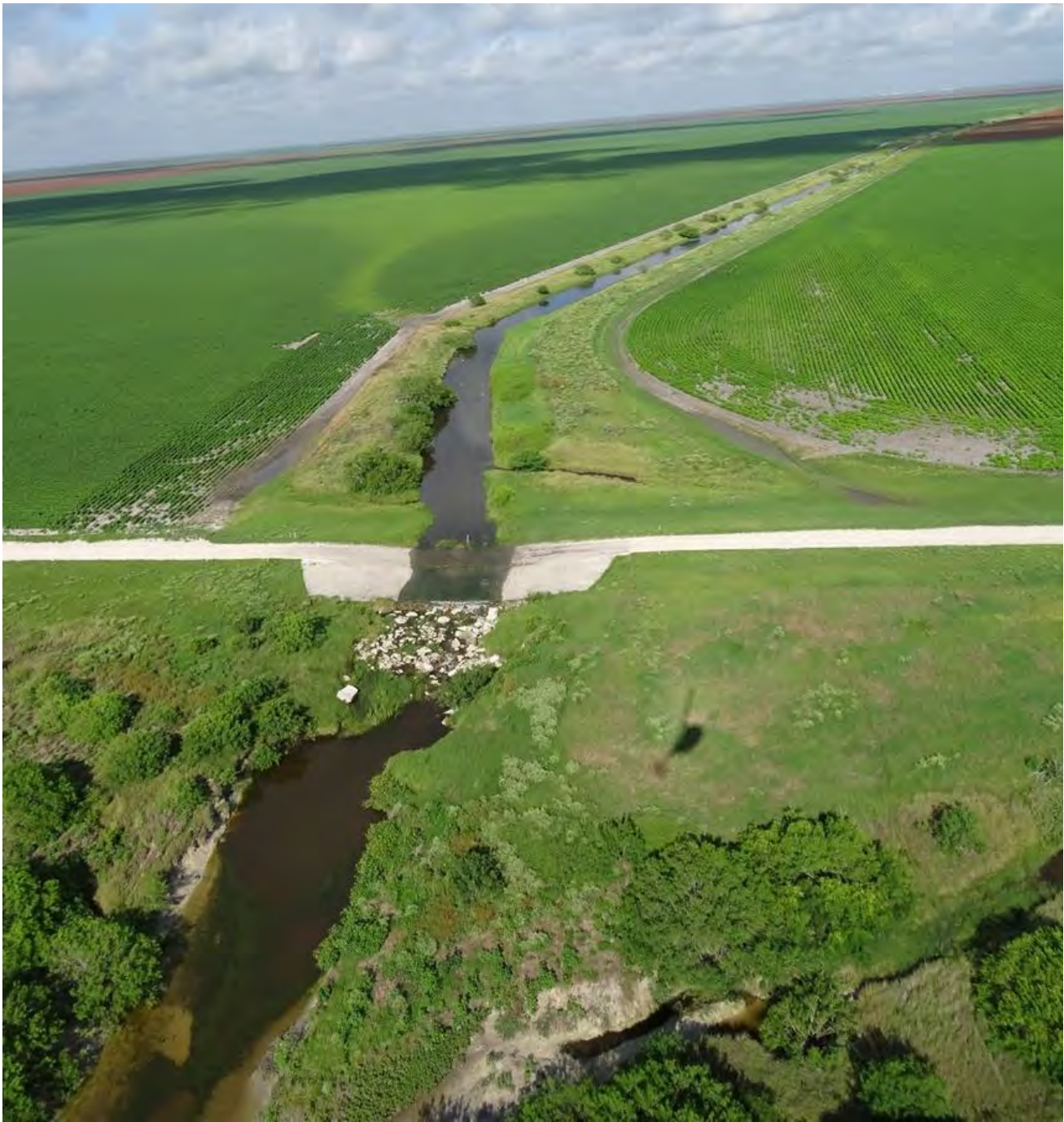
Figure 112 Upstream the creek has been channelized and is more ditch like, straight and narrow. Still the riparian area is marginally functional and well vegetated. Farming activities are beginning to encroach on the creek and its floodplain. The poorly designed crossing pictured here is acting as a gradient control structure and is a source of erosive energy evidenced by a scour pool and head cut.
