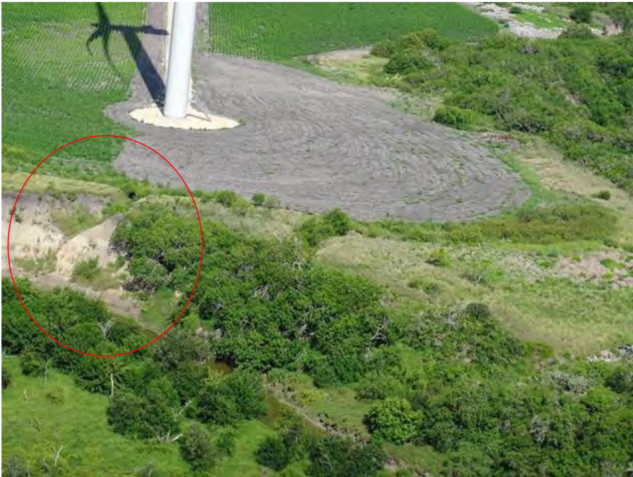
Figure 74 Wind-farm development too close to the creek can also hinder riparian recovery by increasing and focusing runoff. This image shows the bank erosion apparently as a result of enhanced runoff from a tower cited too close to the creek bank without an adequate buffer.
