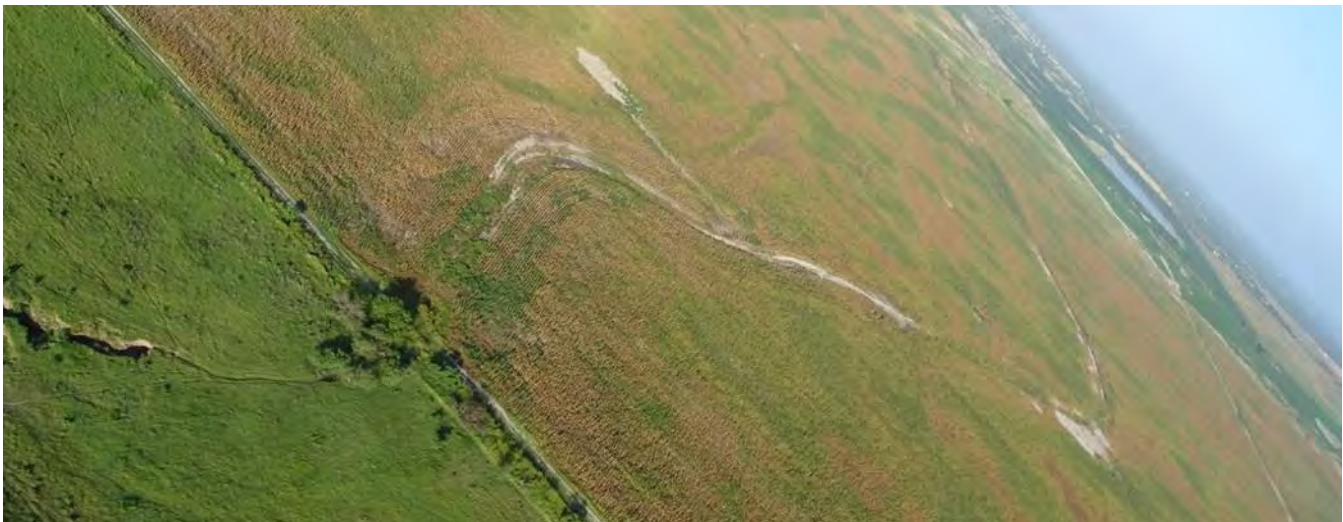
Figure 46 Looking west at Trib A to Radicha Creek south of FM 2220. This image illustrates the hindrance of farming too close to a drain way and the opportunity for enhanced function with a setback of disturbance.
