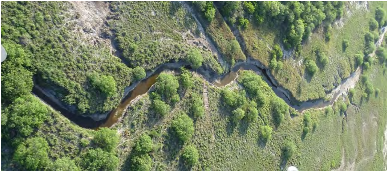
Figure 40 Image shows channel slightly incised and grazing concentrations in the creek area that appears to be hindering vegetation recovery.
