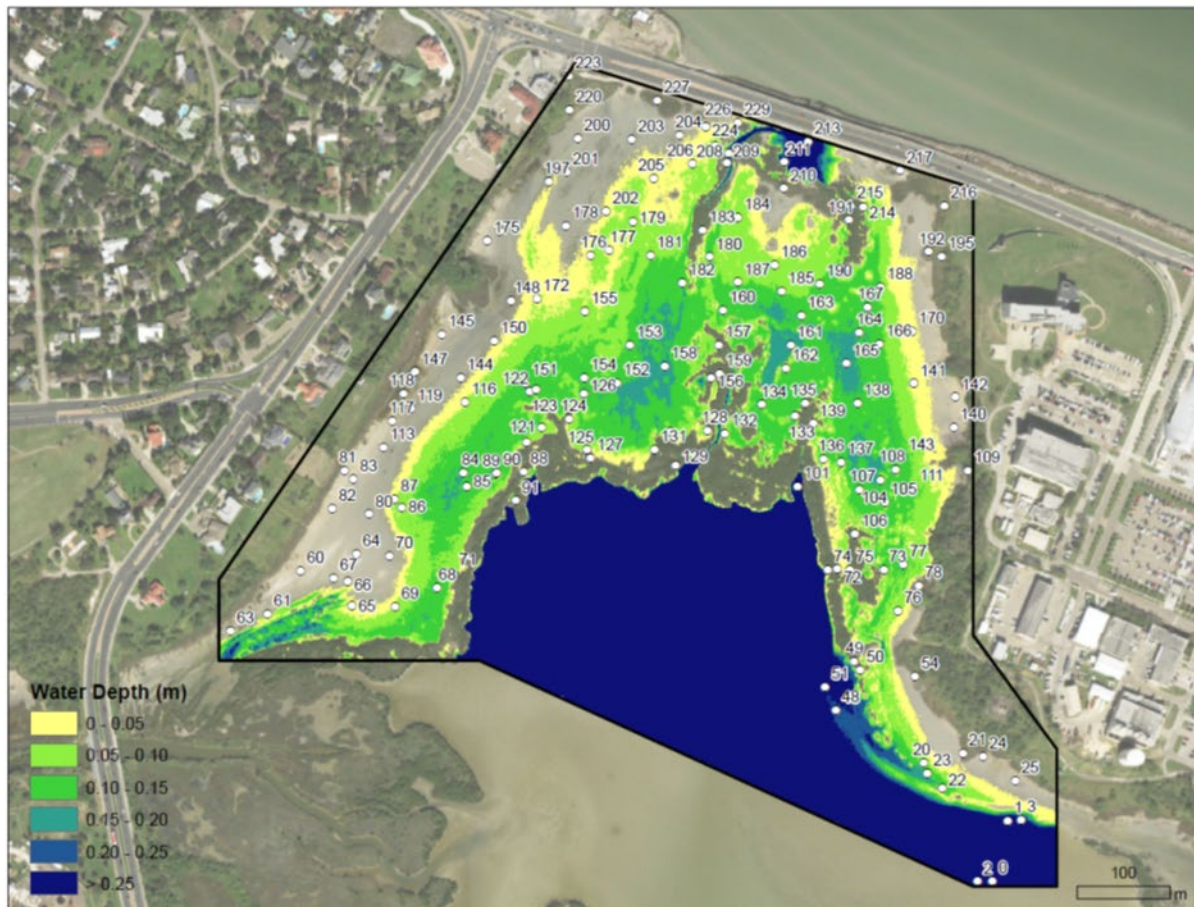
Figure 2. Map of water depths overlain with the points that were ground-truthed during June 2020 to produce the vegetation map. Data collected from these points included ~water depth, and sediment type, and vegetation type.
