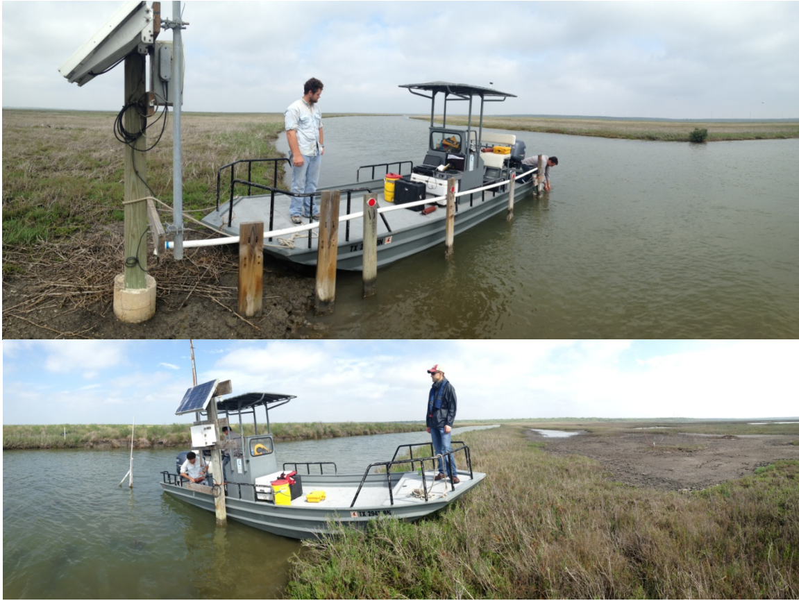
Figure 4. SALT08 (top image) and NUDE3 (bottom image) datasondes are being exchanged with a newly calibrated datasonde which will remain deployed for approximately 4 weeks after which the datasonde will be replaced in the same fashion.
