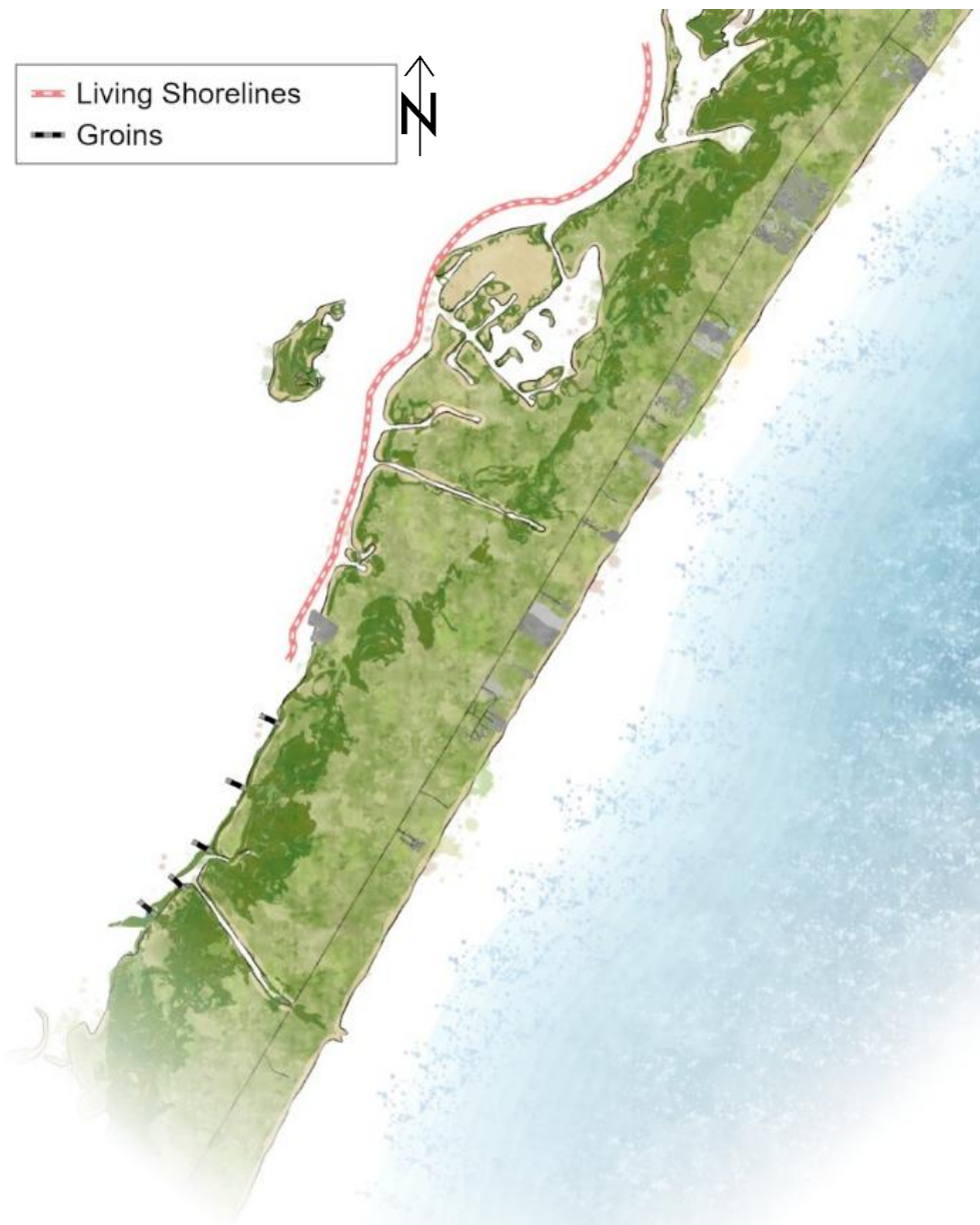
Figure 24 Zoomed-in map to the midsection of Mustang Island showing modeled groins and living shoreline
