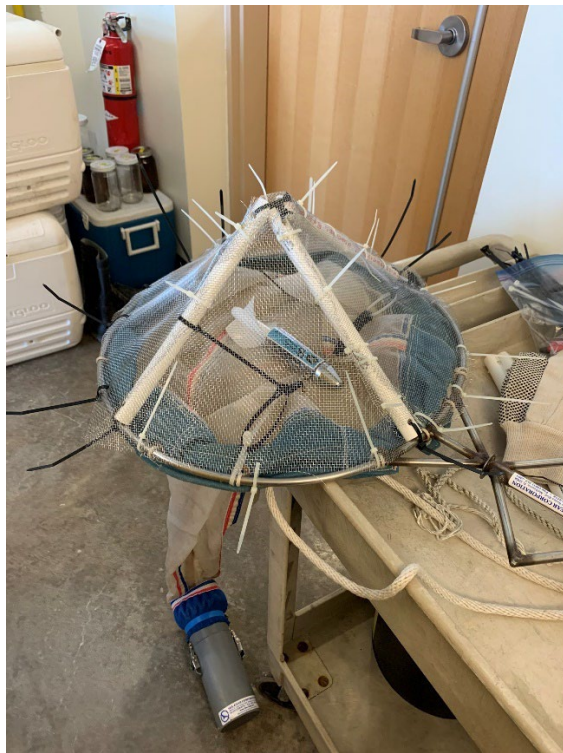
Figure 3. Jellyfish excluder added to bongo plankton net
