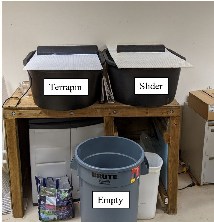
Figure 2. Laboratory tanks used to test the transfer of DNA from live turtle specimen to the water and the degradation of eDNA including a bin without any turtles physically present in the water (Empty).
