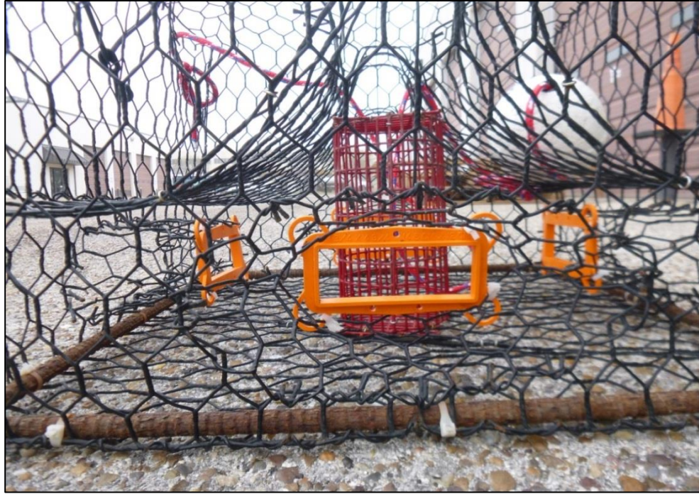
Figure 3. Crab trap fitted with four bycatch reduction devices (BRDs).
