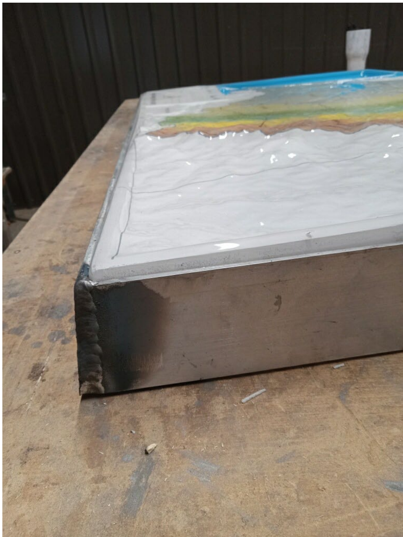
The model is mounted on an aluminum frame for support
