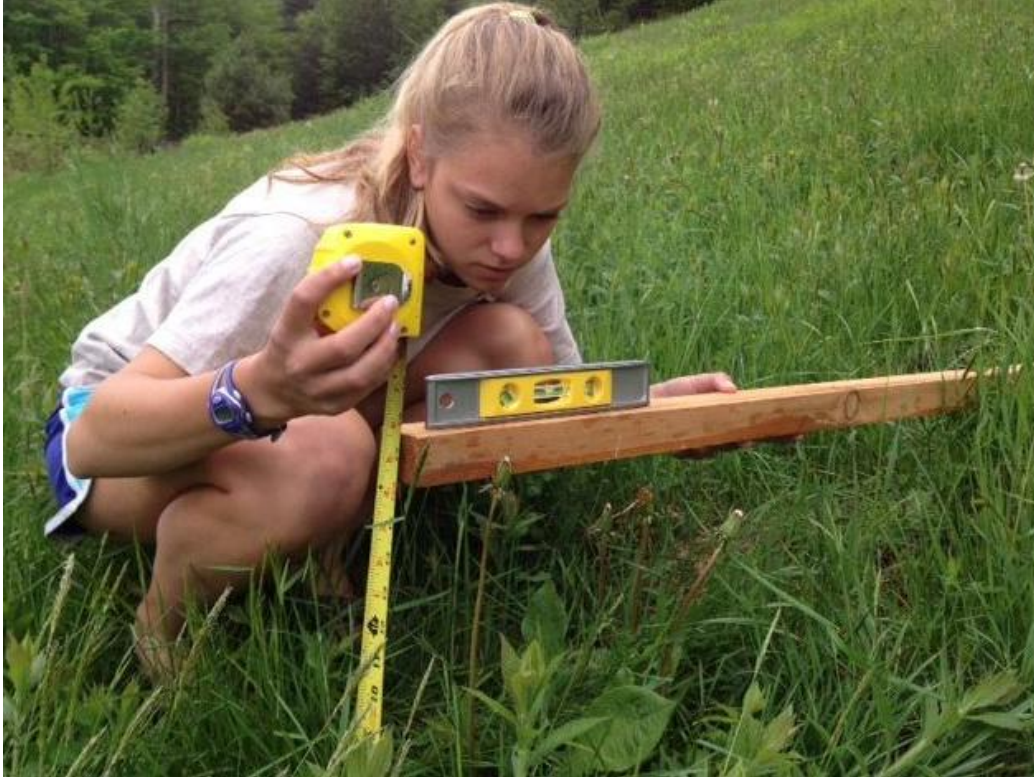
Figure 15. Example of the tape and level slope method ( www.watershedmanagement.vt/gov ).
