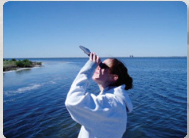
Measuring salinity using a refractometer.
