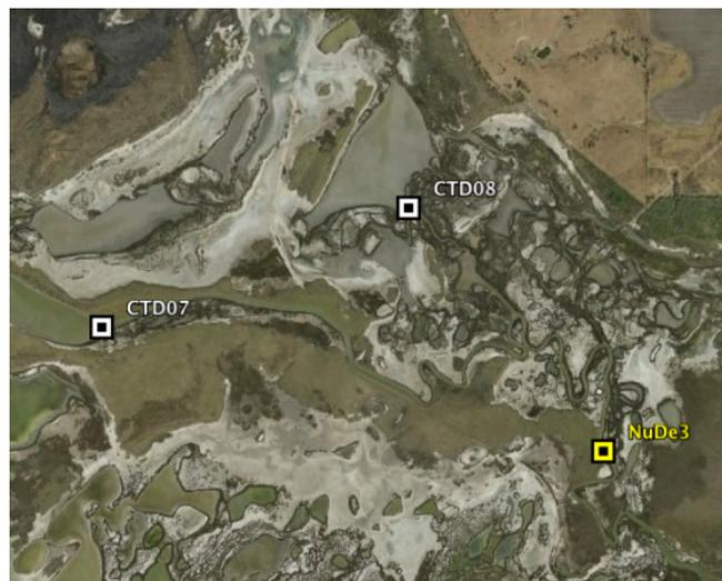
**Figure A.28. Sensors to evaluate fluxes north of main channel. (Google Earth)**
