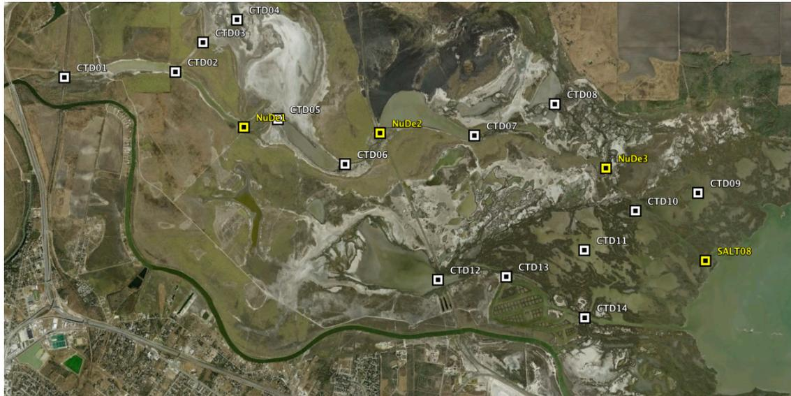
**Figure A.23. Overview of proposed sensor network for calibration and validation. CTD01 through CTD14 are new Conductivity-Temperature-Depth sensors. NuDe1, NuDe2, NuDe3 and SALT08 are existing sensors. (Google Earth)**
