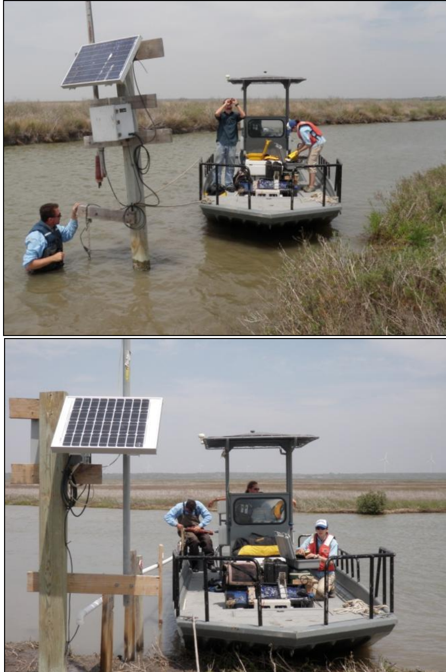
Figure 5. Dominic Burch exchanges the sondes (NUDE3 on top; SALT08 on bottom) with a newly calibrated device, which will last approximately 4 weeks until another sonde will be exchanged again.
