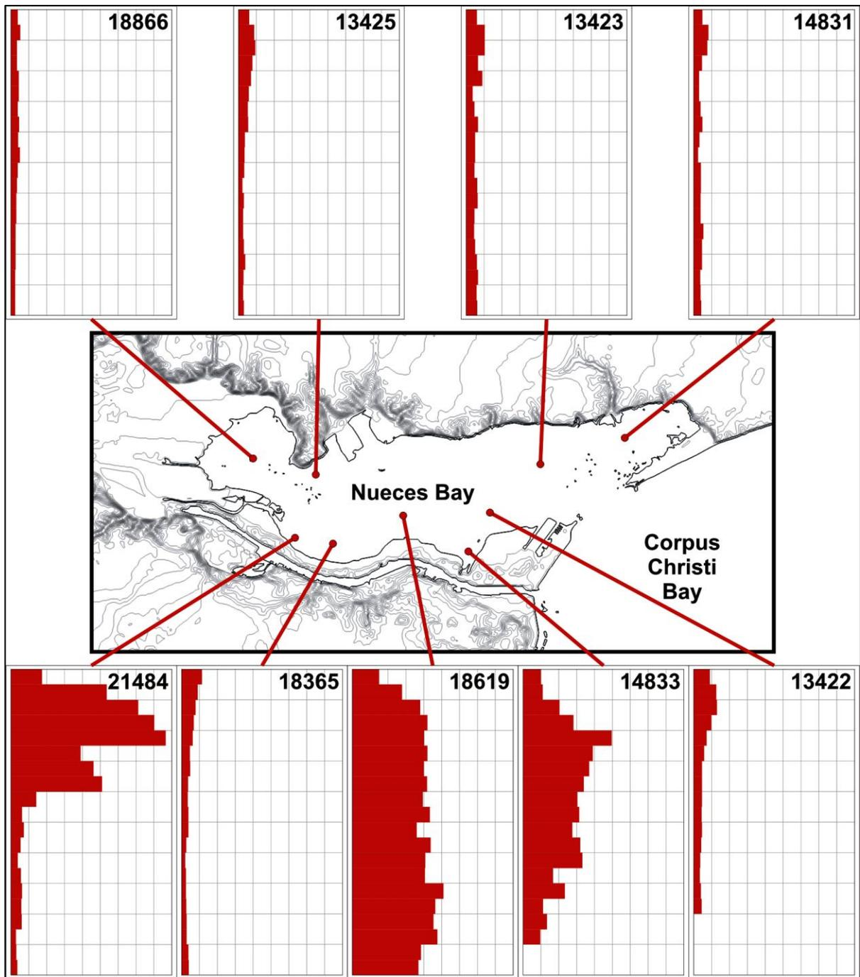
Figure 25. Zinc concentration profiles for Nueces Bay sediment cores from 0-100 cm depth. The horizontal scale for all nine plots is identical, and ranges from 0-450 mg/kg. The graticules mark increments of 10 cm in the vertical direction, and 50 mg/kg in the horizontal direction. The profiles have a blocky appearance because samples were analyzed in 5 cm stratigraphic intervals.
