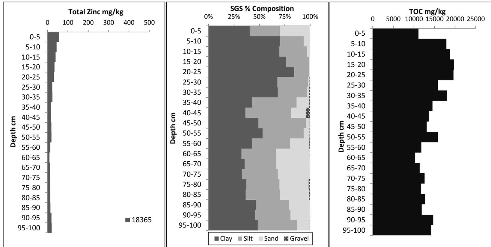
Figure 13. Station 18365 total zinc, sediment grain size, and TOC content in sediment.
