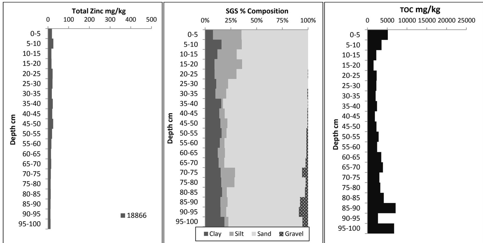
Figure 9. Station 18866 total zinc, sediment grain size, and TOC content in sediment.
