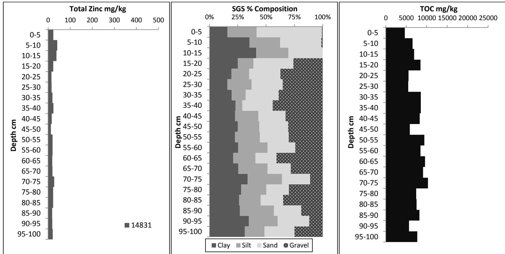
Figure 6. Station 14831 total zinc, sediment grain size, and TOC content in sediment.
