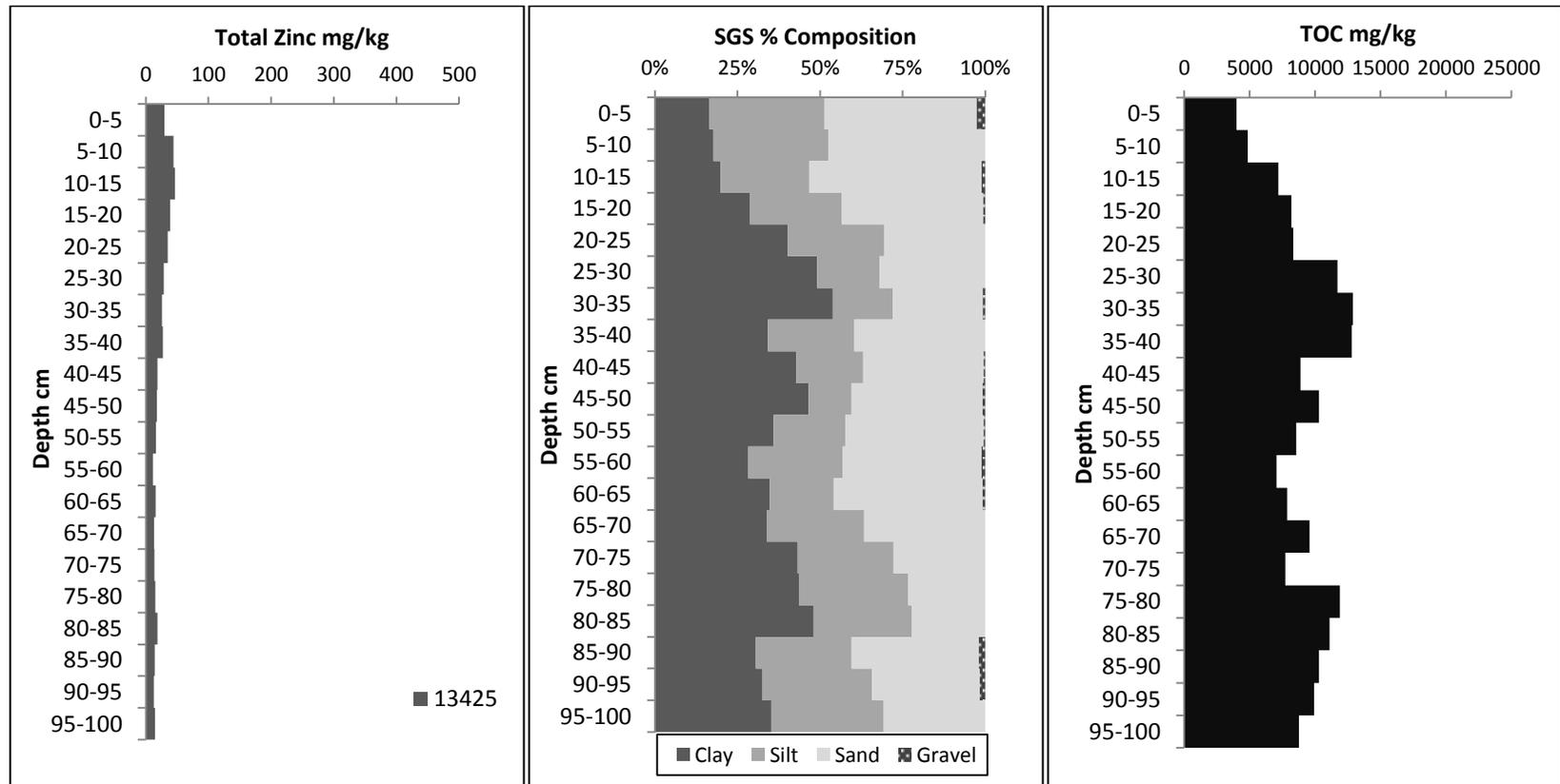
Figure 10. Station 13425 total zinc, sediment grain size, and TOC content in sediment.
