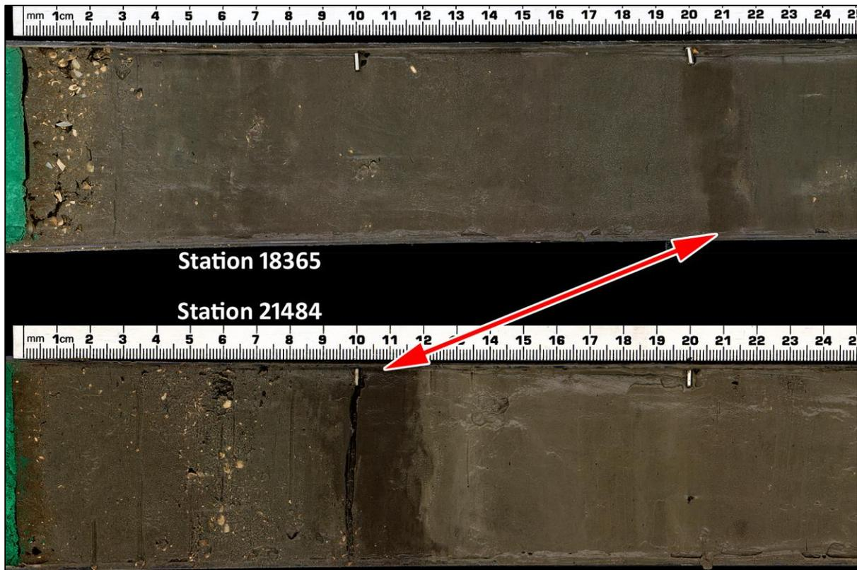
Figure 17. Visual comparison between the upper 0-25 cm of cores from Stations 21484 and 18365. The distinct brown mud band in the 21484 core is found ~10 cm higher in the stratigraphy. This observation supports the assertion that the sediments at Station 21484 may have been disturbed, and may be truncated by ~10 cm (or more).
