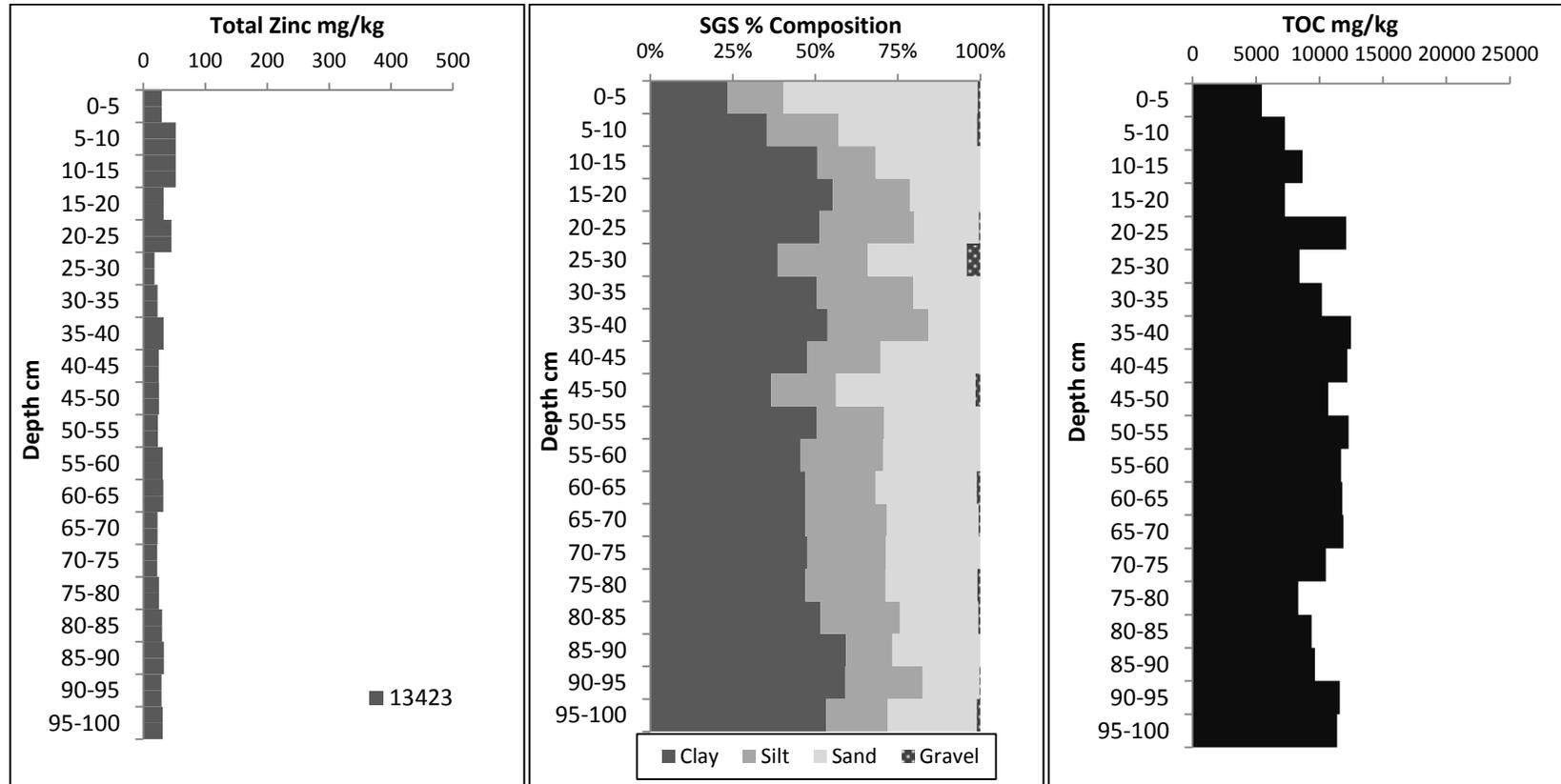
Figure 7. Station 13423 total zinc, sediment grain size, and TOC content in sediment.
