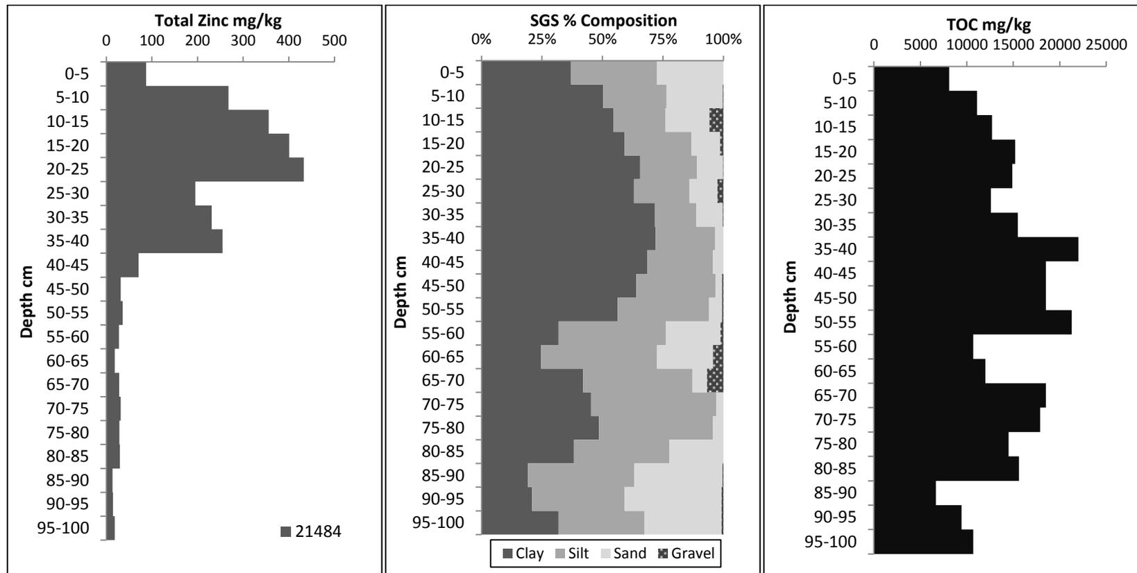
Figure 5. Station 21484 total zinc, sediment grain size, and TOC content in sediment.
