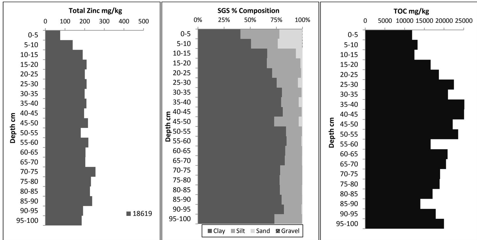
Figure 12. Station 18619 total zinc, sediment grain size, and TOC content in sediment.
