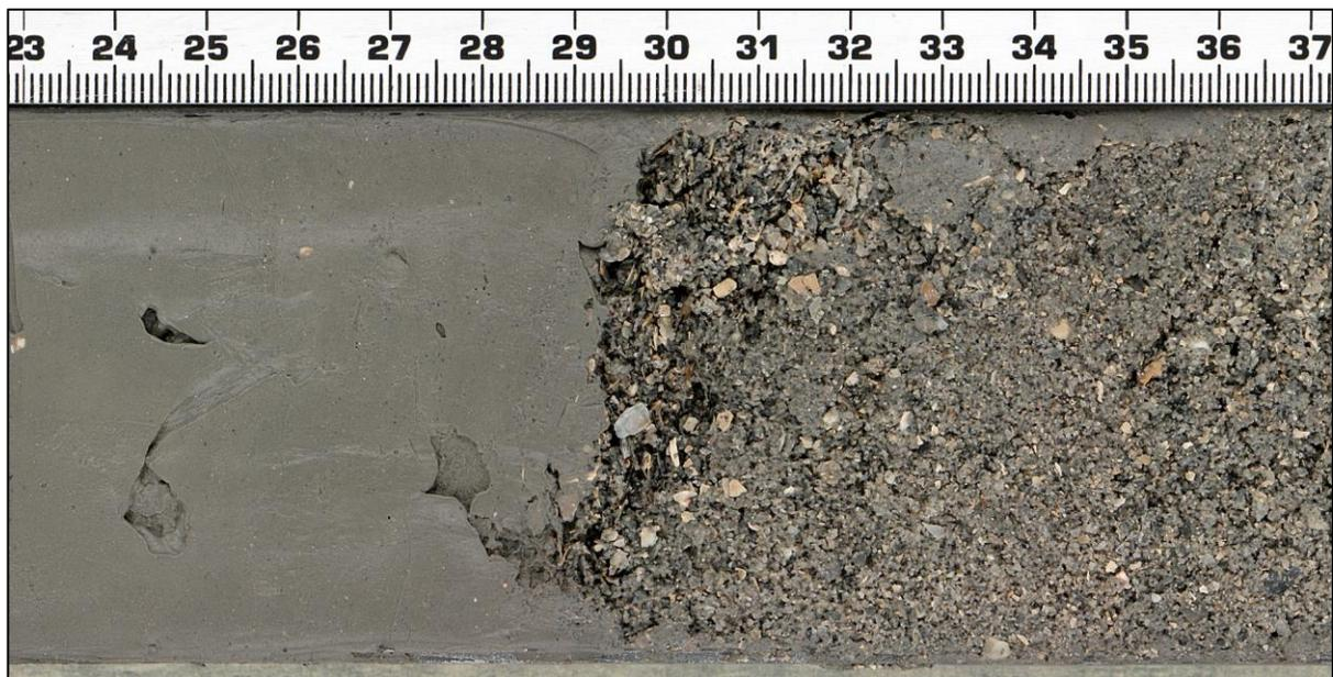
Figure 26. Abrupt transition from shell hash to mud at ~130 cm depth in the sediment core from Station 18619. This abrupt transition, together with a muted magnetic susceptibility profile, relatively constant zinc concentration values down the length of the cores, and the observations made while coring, suggest that this location is a former shell dredge pit or channel that was subsequently filled in rather rapidly.
