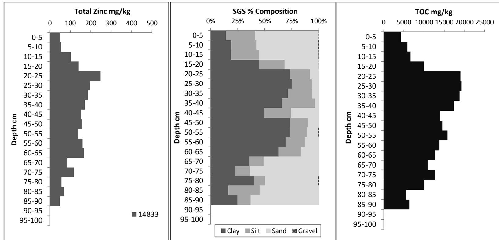
Figure 11. Station 14833 total zinc, sediment grain size, and TOC content in sediment.
