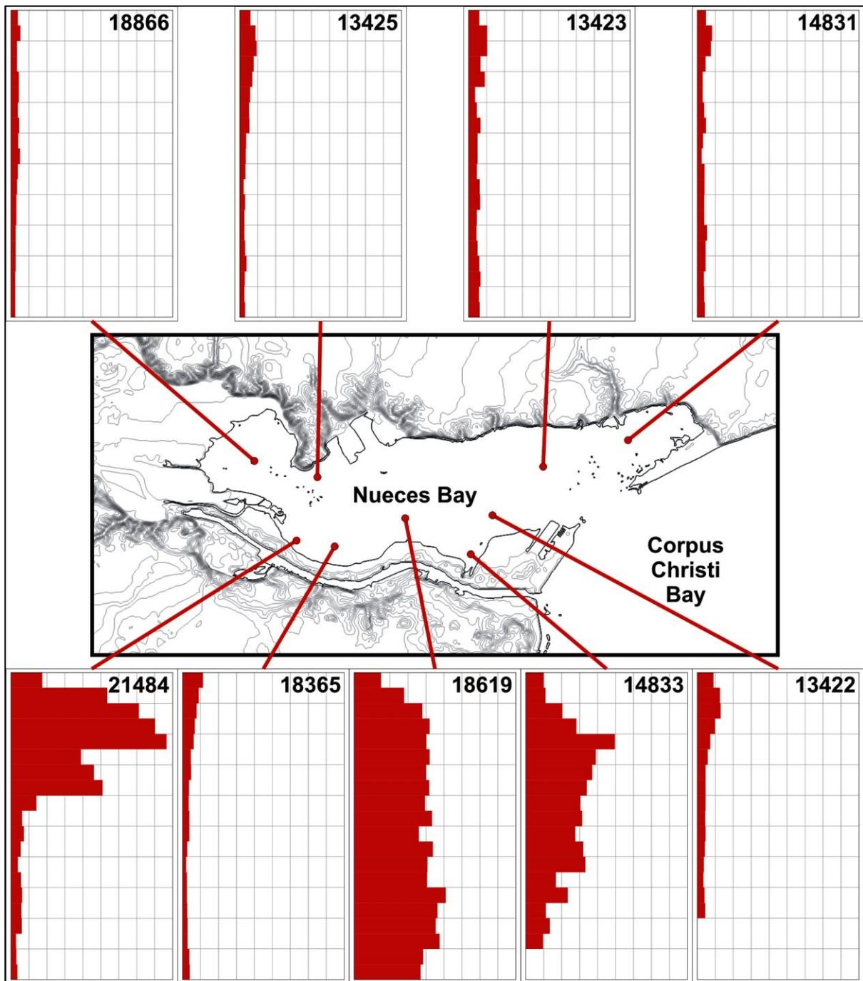
Figure ES 2. Zinc concentration profiles for Nueces Bay sediment cores from 0-100 cm depth. The horizontal scale for all nine plots is identical, and ranges from 0-450 mg/kg. The graticules mark increments of 10 cm in the vertical direction, and 50 mg/kg in the horizontal direction. The profiles have a blocky appearance because samples were analyzed in 5 cm stratigraphic intervals.
