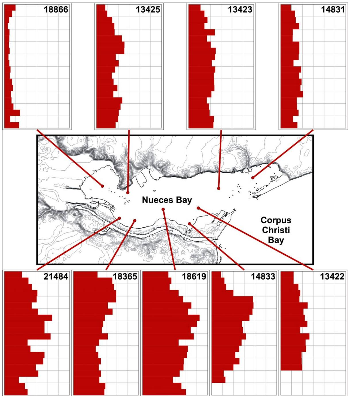
Figure 24. Total organic carbon concentration profiles for Nueces Bay sediment cores from 0-100 cm depth. The horizontal scale for all nine plots is identical, and ranges from 0-30,000 mg/kg. The graticules mark increments of 10 cm in the vertical direction, and 5,000 mg/kg in the horizontal direction. The profiles have a blocky appearance because samples were analyzed in 5 cm stratigraphic intervals.
