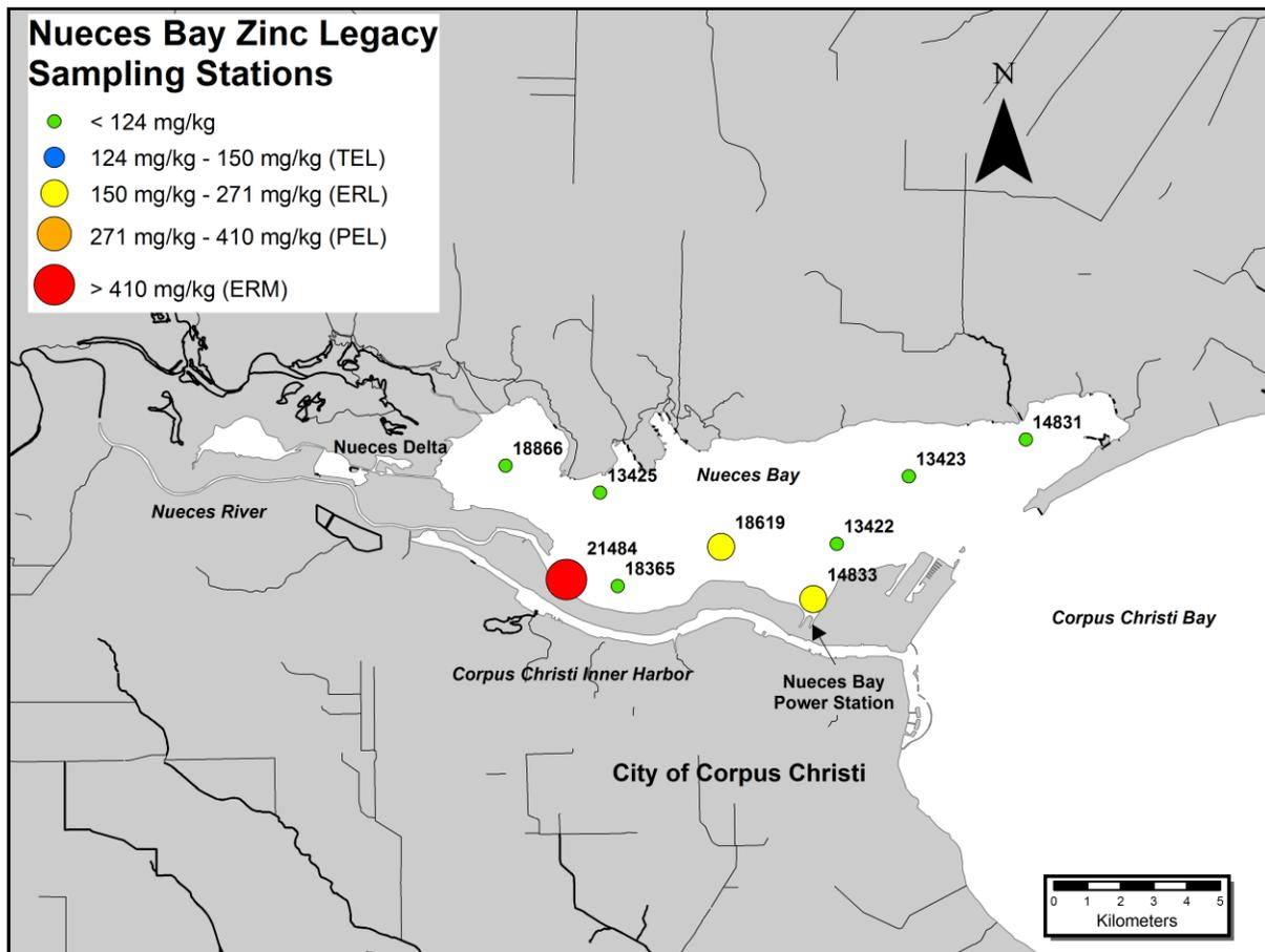
Figure 14. Maximum concentration of zinc in sediment (mg/kg) collected from Nueces Bay sediment profile assessment.
