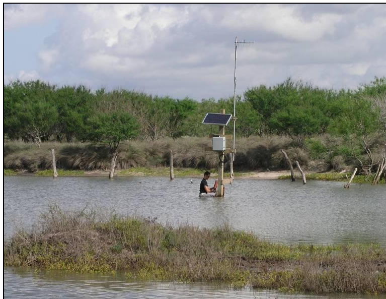
Fig. 3. Field personnel exchanging a datasonde at NUDE01.
