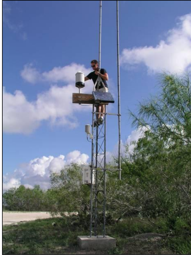
Fig. 6. Real time NUDEWX weather station serviced by CBI field personnel.
