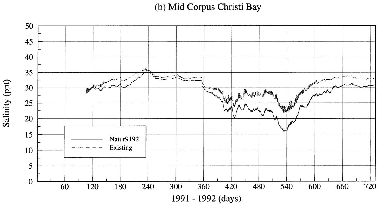
Figure IV.30 Simulated salinities in 1991-1992 for the existing condition and for the all impacts removed scenario
