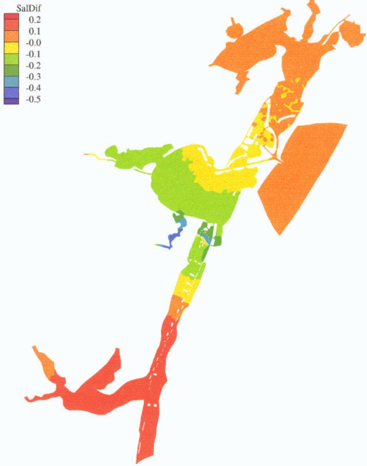
Figure IV.21 Salinity differences (ppt) in August 1989 between the existing and the JFK Causeway removal cases
