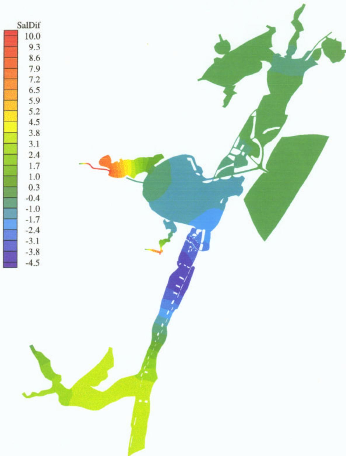
Figure IV.31 Salinity differences (ppt) in August 1989 between the existing condition and the all impacts removed case
