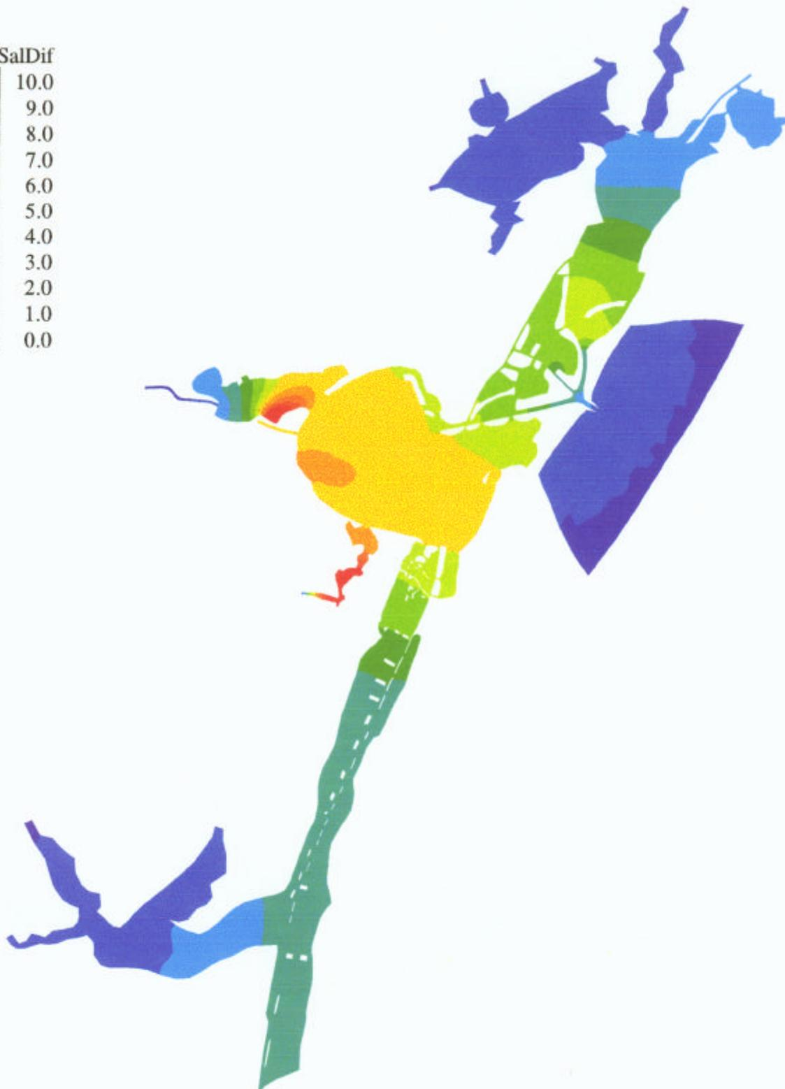
Figure IV.32 Salinity differences (ppt) in May 1992 between the existing condition and all impacts removed case
