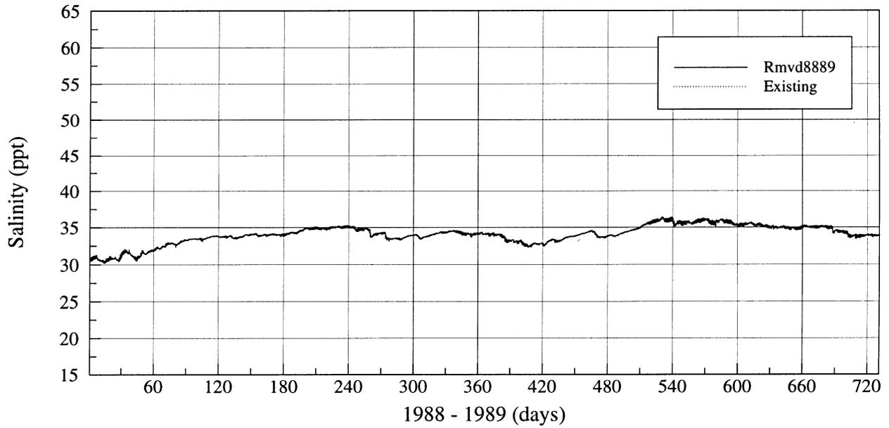
Figure IV.19 Simulated salinities in 1988-1989 for the existing condition and for the JFK Causeway removal scenario
