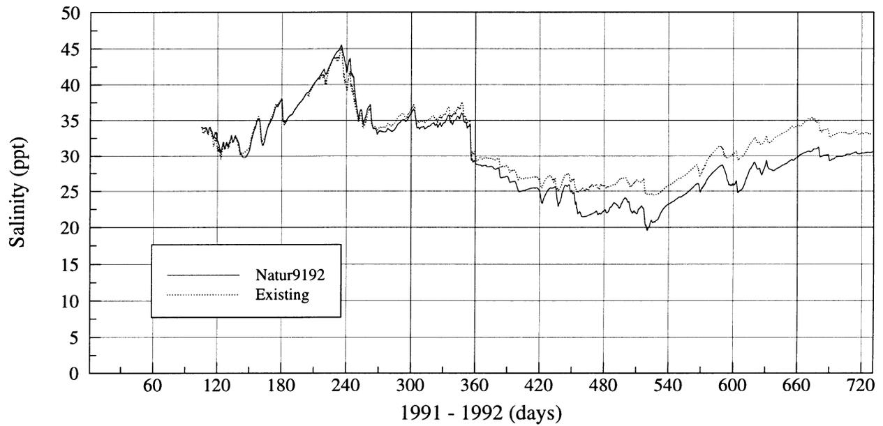
Figure 4.30 Simulated salinities in 1991-1992 for the existing condition and for the all impacts removed scenario
