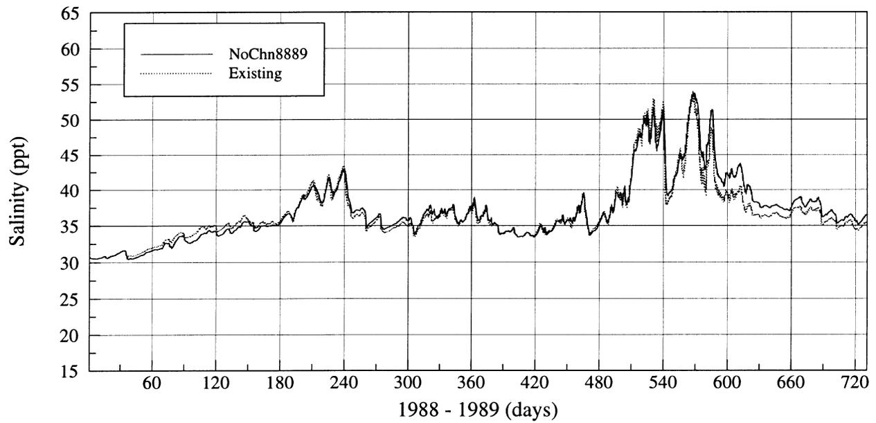
Figure IV.24 Simulated salinities in 1988-1989 the existing condition and for the Corpus Christi Ship Channel removal scenario
