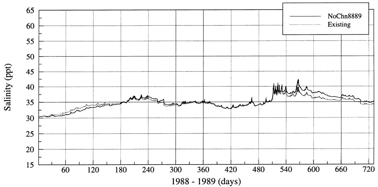
Figure IV.24 Simulated salinities in 1988-1989 for the existing condition and for the Corpus Christi Ship Channel removal scenario
