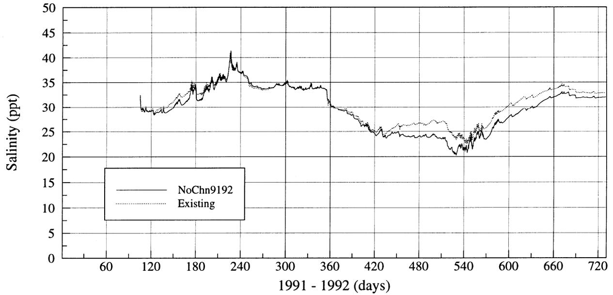
Figure IV.25 Simulated salinities in 1991-1992 for the existing condition and for the Corpus Christi Ship Channel removal scenario
