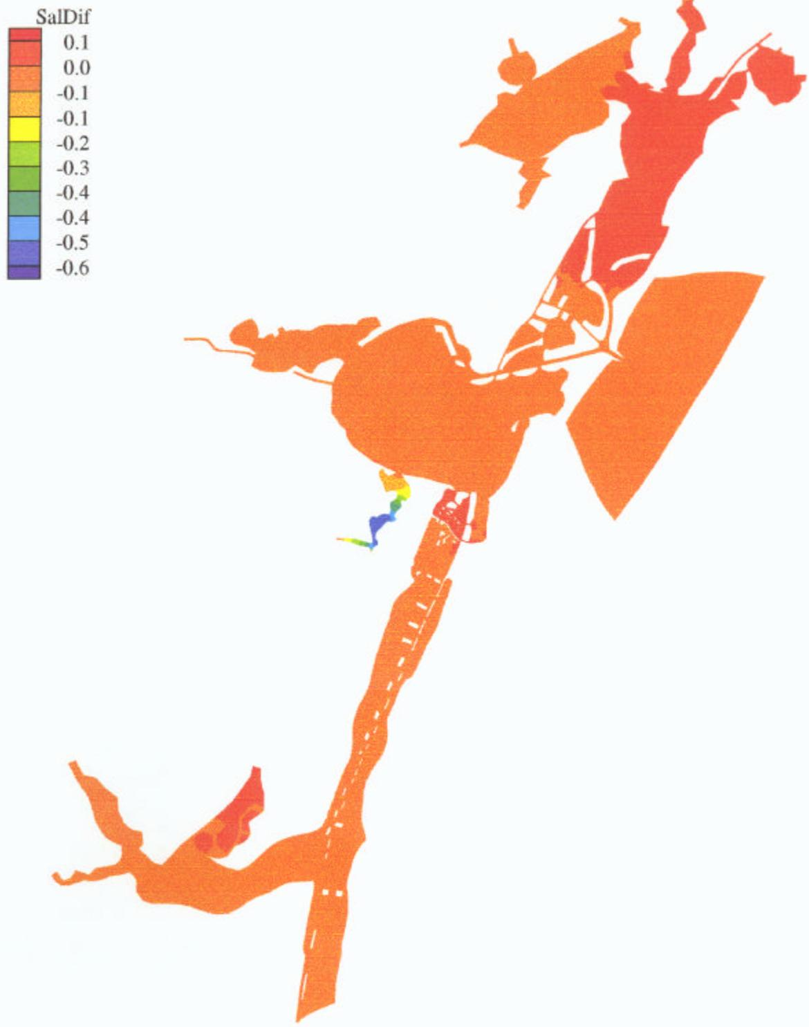
Figure IV.22 Salinity differences (ppt) in May 1992 between the existing and JFK Causeway removal cases
