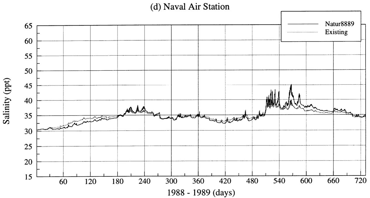
Figure IV.29 Simulated salinities in 1988-1989 for the existing condition and for the all impacts removed scenario
