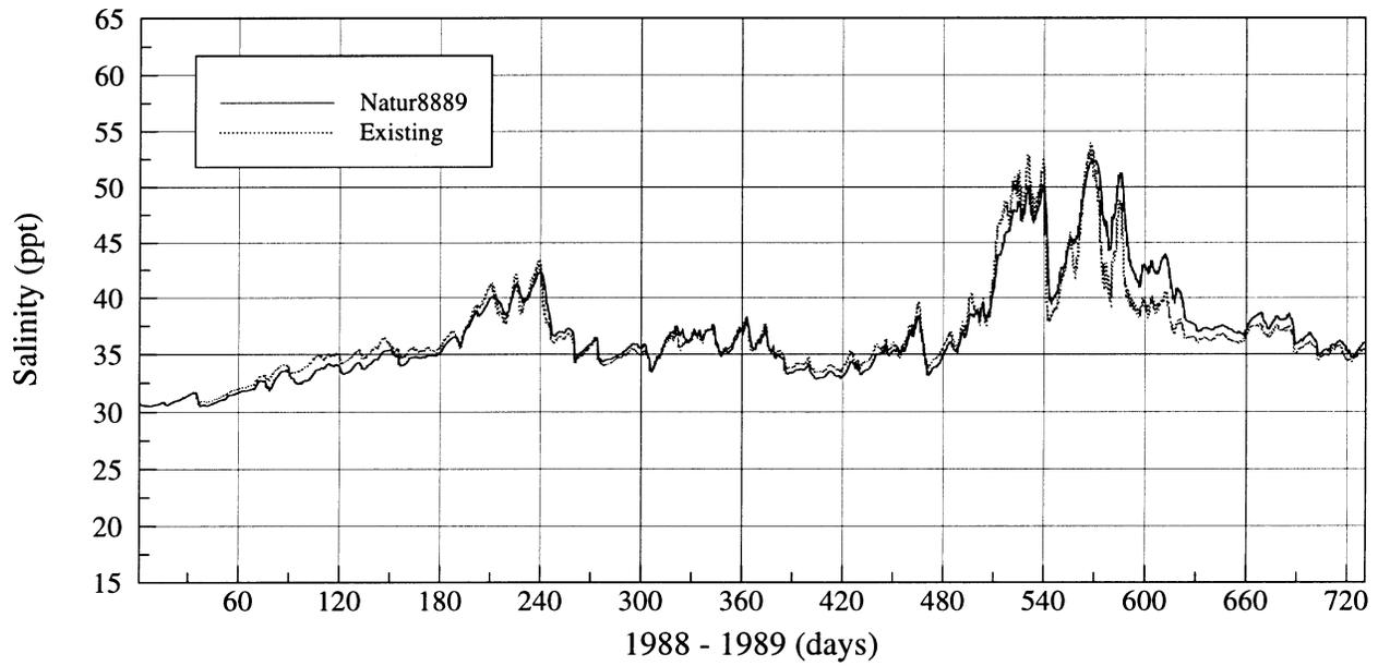
Figure IV.29 Simulated salinities in 1988-1989 for the existing condition and for the all impacts removed scenario
