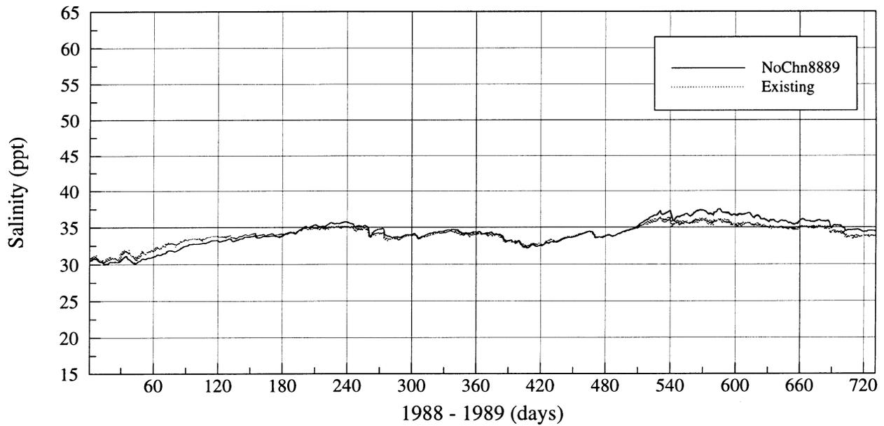
Figure IV.24 Simulated salinities in 1988-1989 for the existing condition and for the Corpus Christi Ship Channel removal scenario
