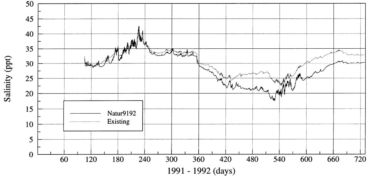
Figure IV.30 Simulated salinities in 1991-1992 for the existing condition and for the all impacts removed scenario
