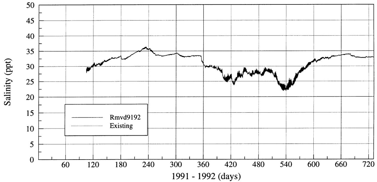
Figure IV.20 Simulated salinities in 1991-1992 for the existing condition and for the JFK Causeway removal scenario
