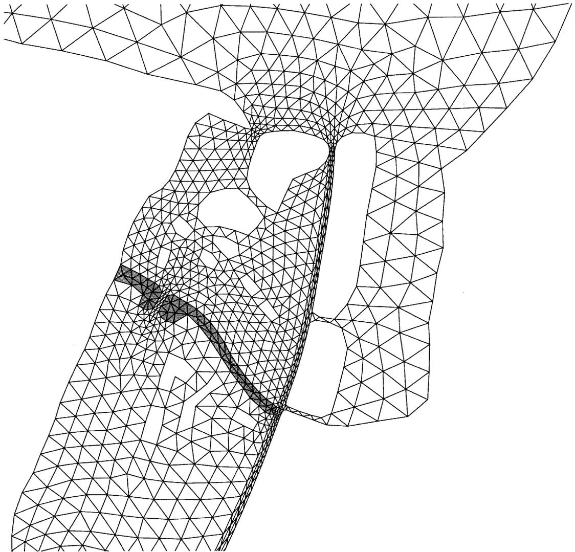
Figure IV.18 Computational grid, focussing on Flour Bluff area, for the JFK Causeway removal case; the shaded elements represent the elevated Causeway elements
